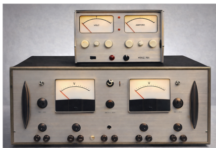
Figure 4: DC laboratory power supplies.
